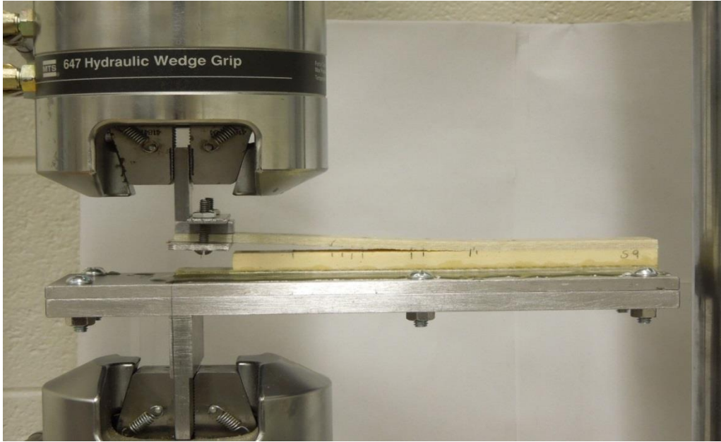
Figure 5.1: T-Peel test setup and SCB sandwich specimen.
